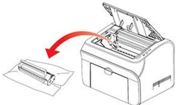
2. Open the package of a new laser toner cartridge, hold the handle of the cartridge and gently shake around 5-6 times, so as to make the toner evenly distributed inside the cartridge.
