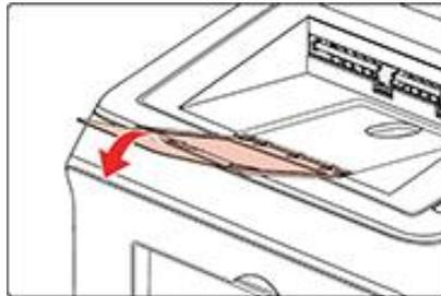
d) Put the print media like an envelope or transparency into the manual feeder tray with two hands until the front end of the envelope or transparency contacts the correction roller.
