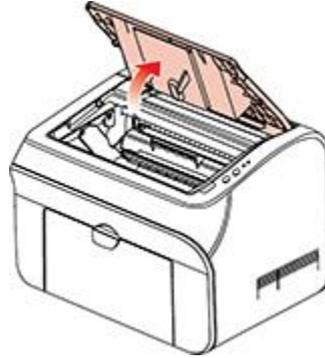
2. Open the upper fuser guide to decrease the pressure of compression spring.
